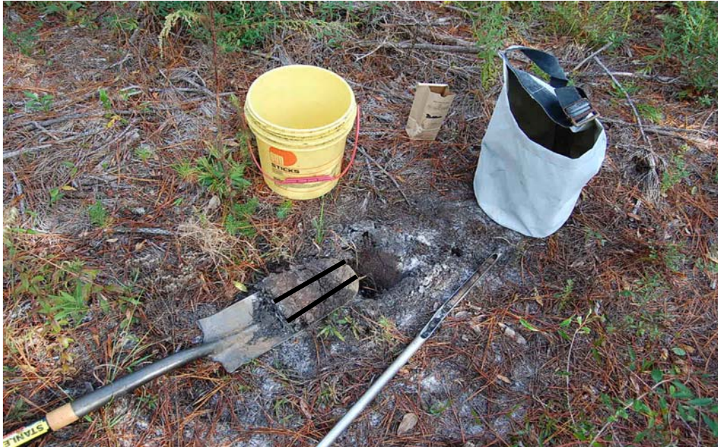
Photo 1. The tools required for soil sampling - clockwise from upper left of photo: a clean plastic bucket, soil bag, planter's bag (or another bucket for carrying several soil samples), soil probe with a 6" soil core, and a narrow shovel with 6" soil sample (only a small vertical slice from the shovel's soil sample will be used per sample location). Make sure each soil bag is filled to the "fill" line.
